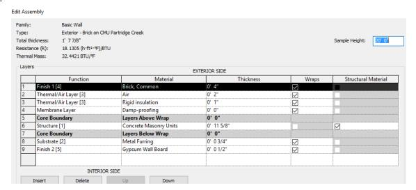
5. Create a Concrete Block wall for the interior portions between two commercial spaces.
