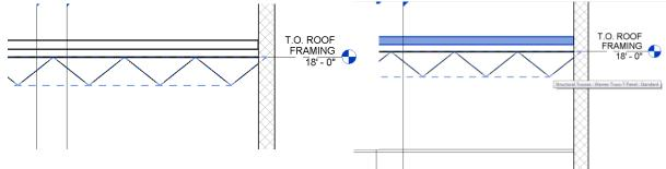
5. Place the roofing deck on top of your truss as shown in the shaded area in the above right picture.
