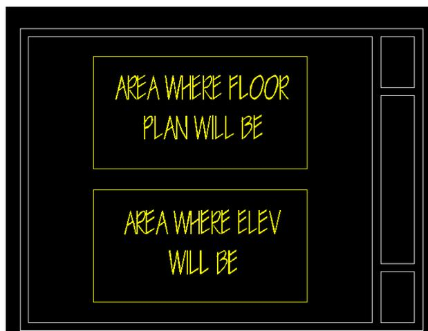
draw a 1/4" drawing. The floor plan and elevation should align, meaning that if you were to strike a vertical line from a first floor window on the elevation it would align with the same first floor window on the floor plan.
