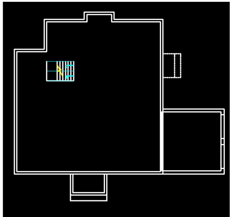
Around the poured basement walls of your basement or porch areas, offset a line 5" in each direction to represent the spread footing. Change this line to HIDDEN and put it on a layer such as the NOTES so it is yellow.
