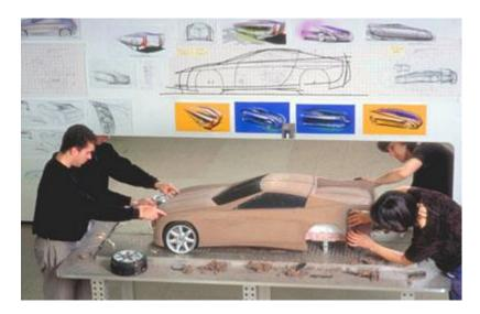
GM modelers use renderings, sketches and tape drawings as reference to create a 1/4 scale half model. Using a mirror in this way enables modelers to produce results more quickly. With full proportioned models, substantial time is spent balancing one side with the other.
