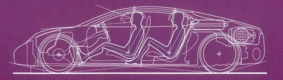
"Without question, the most critical elements in every vehicle package are the occupants. If you get the occupant positions and postures wrong, the entire architecture may need to be redesigned. Because the manikin geometries are constant and represent the customers, the vehicle bodies are scaled around them."
