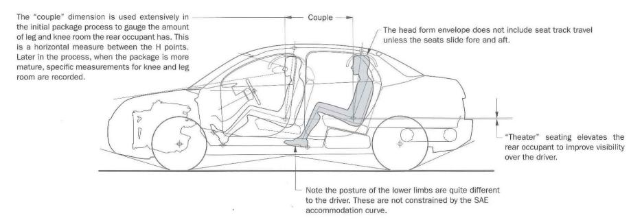
Because the rear occupants do not control the vehicle, their leg posture is not controlled by the accommodation curve. Notice how the knee angle is quite different to the driver and their feet are flat on the floor. Second, the demographics for the rear occupants may be different to the front occupants. They may be children or people who are shorter in stature to the driver, so headroom, for example, may be less.
